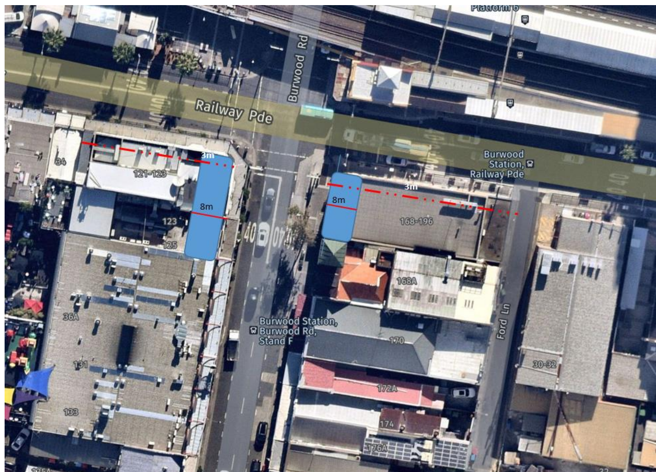
Figure 1. Increased street front setback requirements for 121-125 & 168 Burwood Road, Burwood – 8m setback to Burwood Road and 3m setback to Railway Parade
